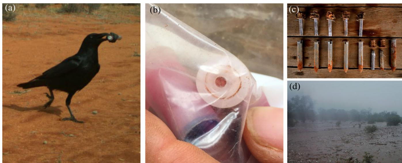
**Figure 1.** (a) Australian corvid (*Corvus* sp.) removing the ejector unit, trigger, poison capsule and lure head from a CPE, (b) degradation of the plastic capsule containing the 1080 poison, (c) corrosion of the CPE units, (d) hail events during the canid pest ejector monitoring and the flooding of wheel ruts on vehicle track and surface water run-off.
