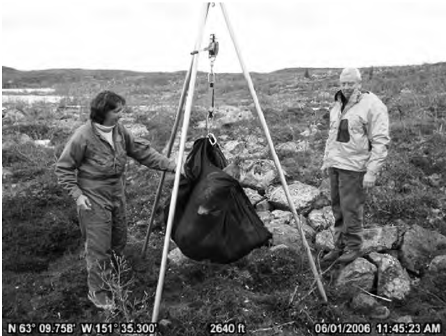
Fig. 6.1 Tripod mounted scale for weighing a brown bear (Pat Owen, NPS, Denali Park and Preserve).
