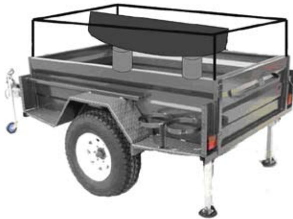
Figure 7: A delivery system such as the ‘Camel Canteen’ would require the height and neck length of a camel to gain access to the ‘bait’ hopper
