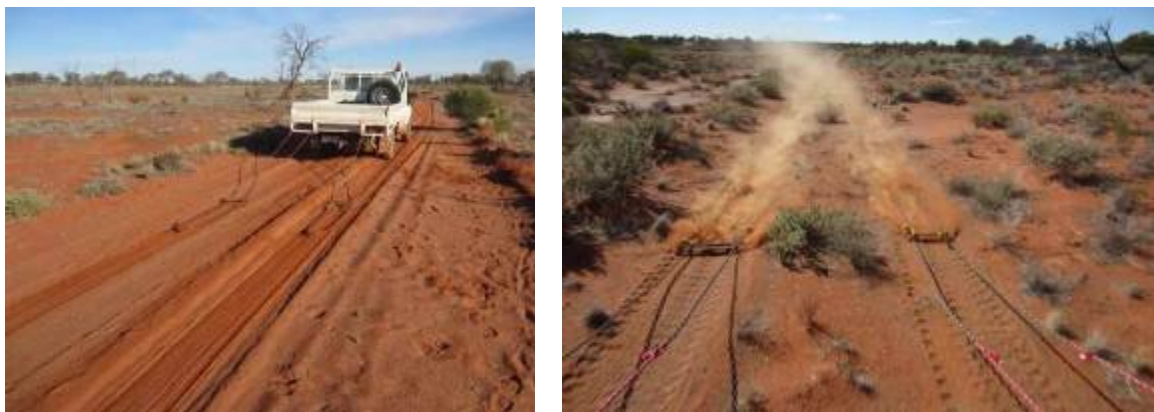
Figure 6. Apparatus used to smudge tracks after daily counts.
