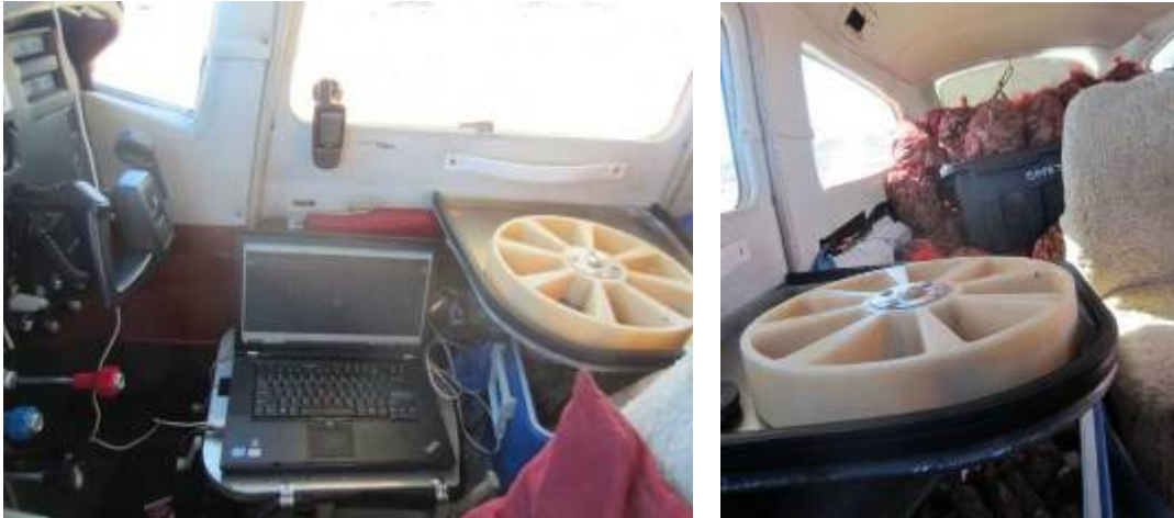
Figure 8. (a) Inside the aircraft: carousel, computer and independent GPS. (b) Baits were stored alongside and behind the bombardier.
