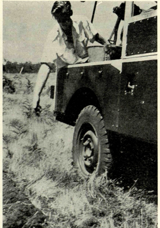
Fig. 4.—Today all the furrow cutting and bait laying done by the Agriculture Protection Board is done mechanically. Here oats are being dropped from a Land Rover into a furrow cut previously by the same vehicle —Photo by C. D. Gooding.
