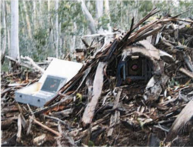
Figure 3.3 Photograph showing placement of thermal imaging camera and laptop in a field situation (Bago State Forest, NSW)
