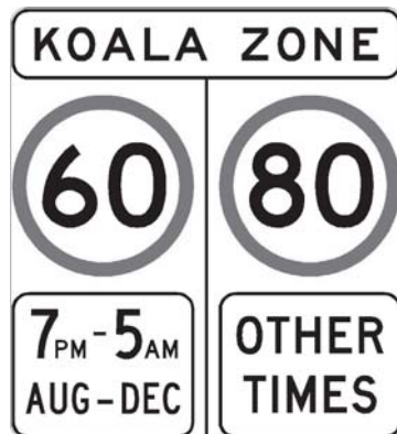
Fig. 3. An example of a differential koala speed-zone sign used during the study.
