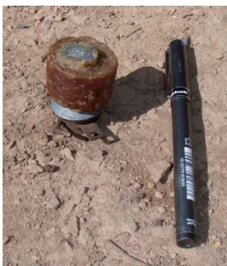
FIGURE 1 A set M-44 ejector. When the target animal pulls on the baited ejector head, a spring-loaded plunger propels through a capsule containing the toxicant (center of the head), discharging the contents into the animal's mouth. (Photograph courtesy of Rob Hunt, NSW DECCW.)
