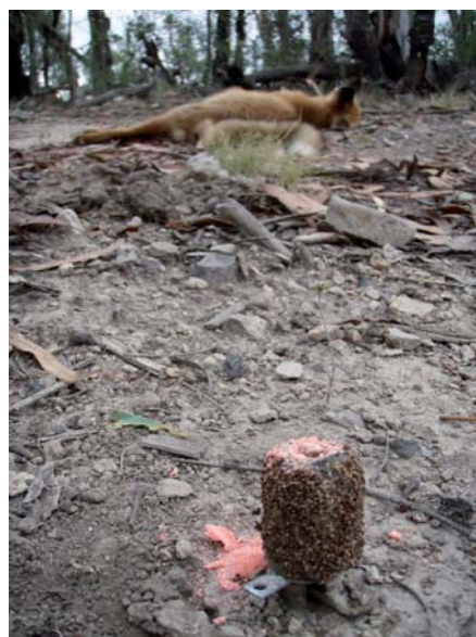
FIGURE 2 A discharged M-44 ejector (foreground) with the carcass of the targeted fox nearby. (Photograph courtesy of Rob Hunt, NSW DECCW.)
