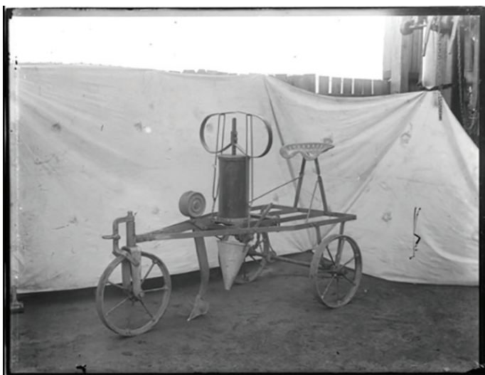
Figure 4: “Toxicon” rabbit poison distributor, made by The Clyde Engineering Co. Ltd, Granville, New South Wales, Australia, 1900-1945. Reg. 88/297-578. Source: Powerhouse Museum
